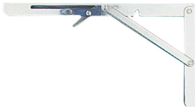
**Description:** Foldable arm pair, for table models 71.202.00; 71.202.60; 71.202.70; made of stainless steel, supplied with a kit for mounting the pipes into post Ø 22/30 mm.
