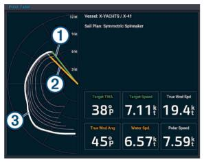
Target wind speed and angle, where the length of the line indicates the speed
