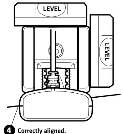
**Adjusting the Horizontal Transducer Angle**
