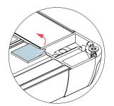
Turn over and remove protective covers from adhesive pads in each corner.
