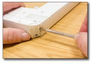
Keeping spring under tension, clip the tensioner back in to the corner moulding.
