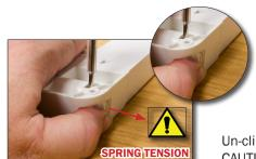
Un-clip the tensioner as shown. CAUTION, this will be under spring tension.
