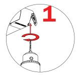
Ensuring mounting surfaces are free form dust or grease, use the adhesive pads to hold the SKYCREEN in position and drill pilot holes. Ensure that the thickness of the boat structure at the proposed mounting position is deep enough to prevent the fixing screws from breaking through. Oceanair recommend No6 x 16mm [5/8"] PANHEAD Screws (not provided). However if necessary, use shorter fixing screws and use masking tape on the drill bit as a depth guide to avoid drilling too deep.
