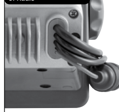
Wiring Located at Back of Radio
