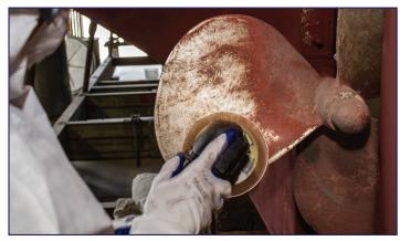
1.2 Sand thoroughly all metallic surfaces with <u>dry</u> sandpaper n. 80, renewing it often. A dual action rotary sander can be used. Do not use wet sandpaper. The surface must be very rough after sanding. Do not use coarser than 80 grit, nor finer, nor worn out sandpaper. Do not use scotch brite. We do not reccomend sandblasting unless done by an experienced professional.
