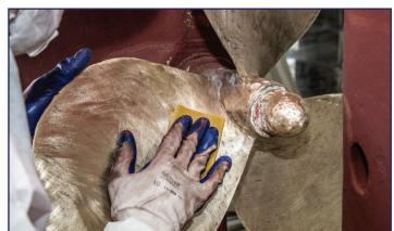
IMPORTANT: All metallic surfaces must be rough and clean. Do not touch the surfaces with bare hands, that may leave traces of grease or dirt. For cleaning grease and dirt use only our SOLVENTE 102 or pure Acetone. Absolutely do not wash the sanded surface with water, soap, detergents, acid!
