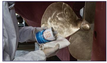
1.3 Wash and degrease carefully all metallic surfaces with our SOLVENT 102 ANTISILICONE (or pure ACETONE) and a clean rag. Change rag frequently, especially in case of new or folding propellers, which usually have more grease on them.
