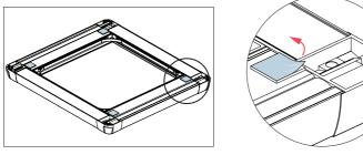
Turn over and remove protective covers from adhesive pads in each corner.
