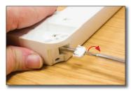
Turn clockwise to tension or anti-clockwise to de-tension. NOTE: No more than 8 full turns should be required.
