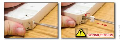
Insert screwdriver in tensioner slot and allow spring to retract from corner moulding. Spring tension will now be felt in the two directions shown.
