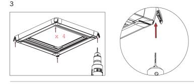
Ensuring mounting surfaces are free form dust or grease, use the adhesive pads to hold the SKYCREEN in position and drill pilot holes. Ensure that the thickness of the boat structure at the proposed mounting position is deep enough to prevent the fixing screws from breaking through. Oceanair recommend No6 x 16mm [5/8"] PANHEAD Screws (not provided). However if necessary, use shorter fixing screws and use masking tape on the drill bit as a depth guide to avoid drilling too deep.
