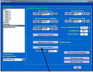
Click on "Scan Port Com GEOS n°11. The program then searches for the GEOS. Due to sensitivity, it may not find the GEOS on the first try. Re-try the Scan Port.
