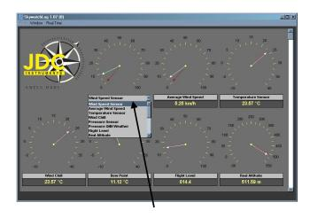
The "Console" view will display the measurements on weather dials. Select what is displayed on each dial by selecting from the drop down menus.
