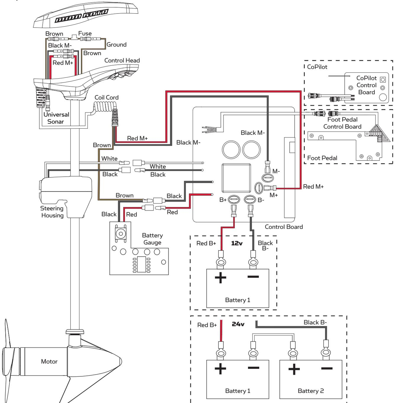
**NOTE:** This is a multi-voltage diagram. Double-check your motor's voltage for proper connections. Over-Current Protection Devices are not shown in this illustration. If equipped with Universal Sonar, please see instruction sheet on the website at [minnkotamotors.com](http://minnkotamotors.com).
