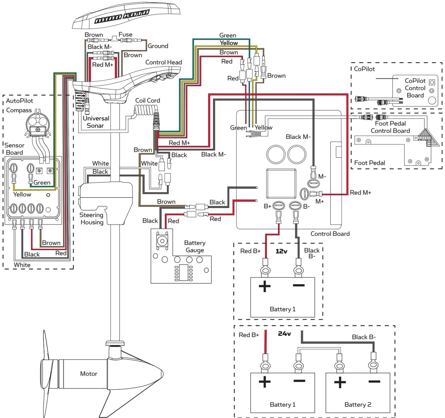
**NOTE:** This is a multi-voltage diagram. Double-check your motor's voltage for proper connections. Over-Current Protection Devices are not shown in this illustration. If equipped with Universal Sonar, please see instruction sheet on the website at [minnkotamotors.com](http://minnkotamotors.com).
