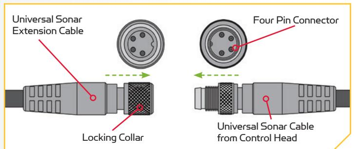
**NOTE:** The connectors are keyed to prevent reversed installation.
