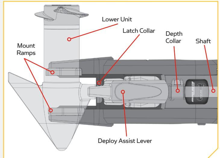
**NOTE:** Slide the Depth Collar down and secure it against the top of the Steering Housing when stowed to secure the motor in place and prevent accidental deployment.
