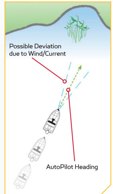
**NOTE:** After steering to a new direction, there is a short delay before the direction is locked in to allow the compass to stabilize. When broad speed changes are made, the AutoPilot heading may change slightly. This is normal.
